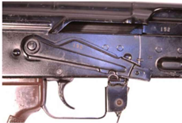
Figure 7. The Selector Lever Placed on SEMI.
