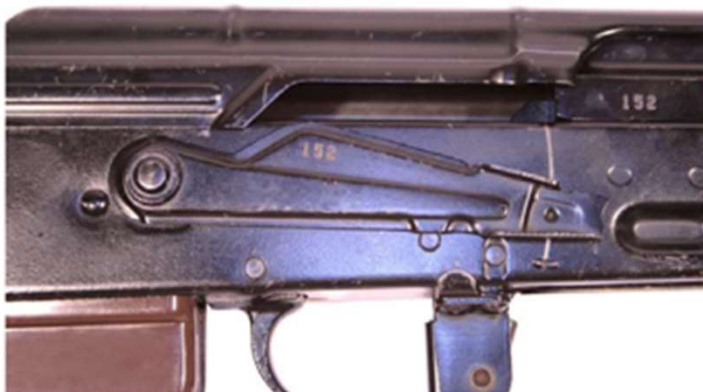
Figure 8. The Selector Lever Placed on AUTO.
