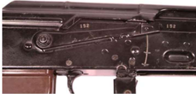
Figure 6. Selector Lever Placed on SAFE.
