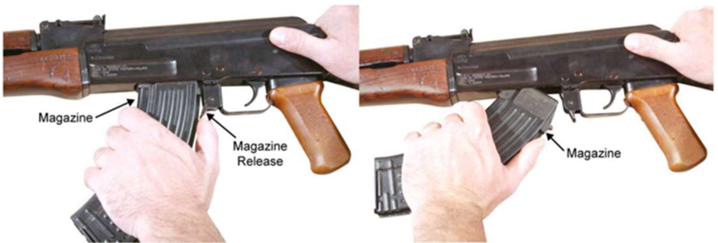
Figure 2. Removing the Magazine.
