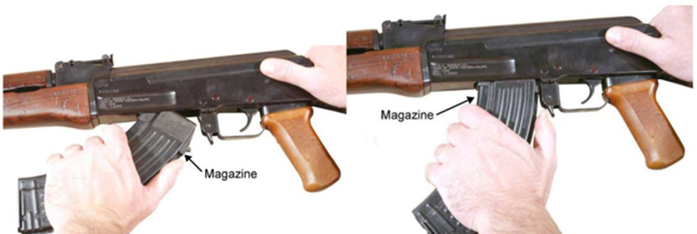
Figure 1. Inserting a Magazine.
